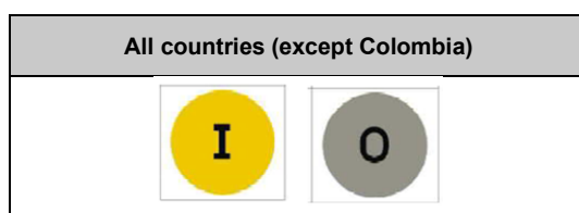
Figure 18 - Indicator for the position of the earthing switch in line functional unit
