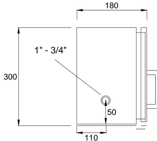
**FIGURA 3 DETALLE BARRAJE PARA ACOMETIDAS: Fases y Neutro**
