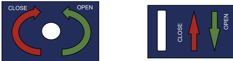
Figure 8– Point for the operation of switch-disconnector in line functional unit
