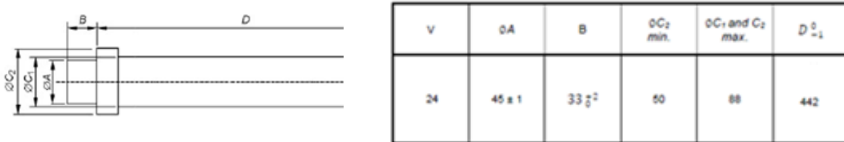
Figure 27 – Fuse-link Dimensions
