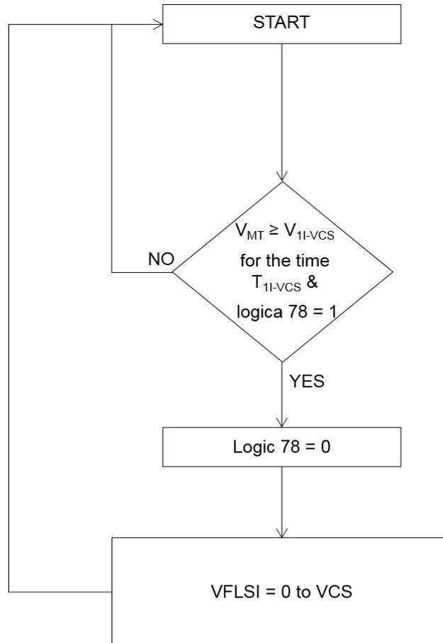
**Figure 11 – logic for the re-entry of the VFLSI to the VCS (logic 8)**
