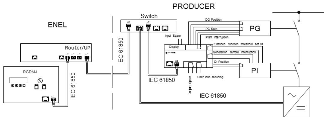
**Figure 2 – DG Interfacing mode**
