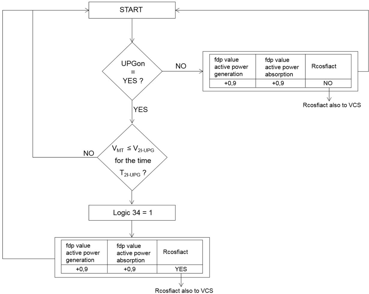
**Figure 6 –Logic for local generation of Q (logic 3)**
