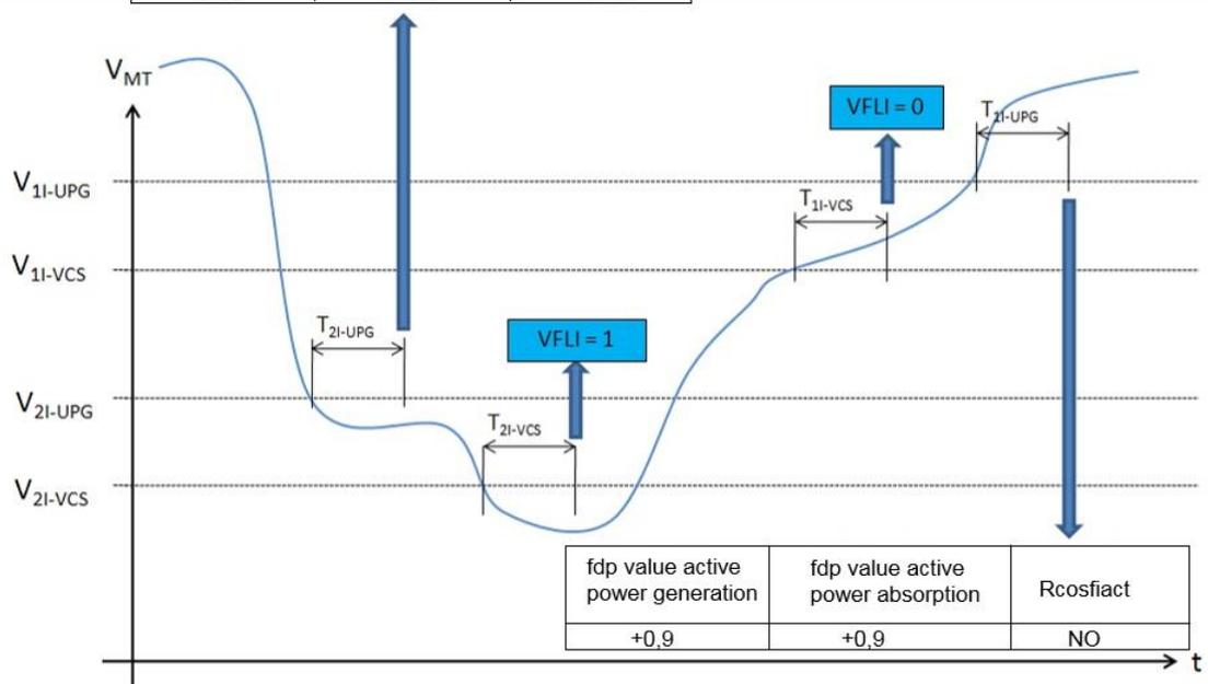
Figure 13 – Threshold for “Low MV Voltage”
