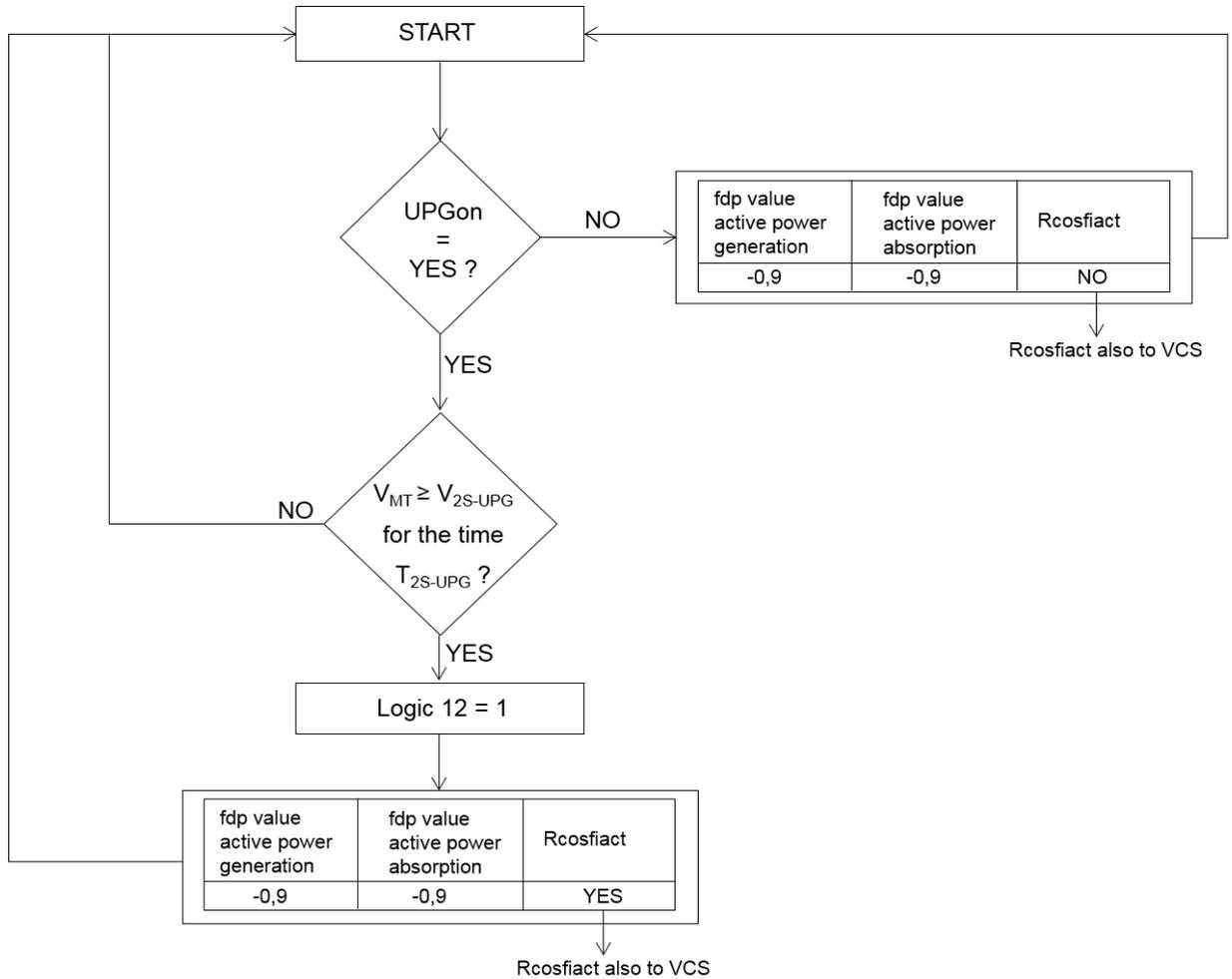
**Figure 4 – Logic for local absorption of Q (logic 1)**
