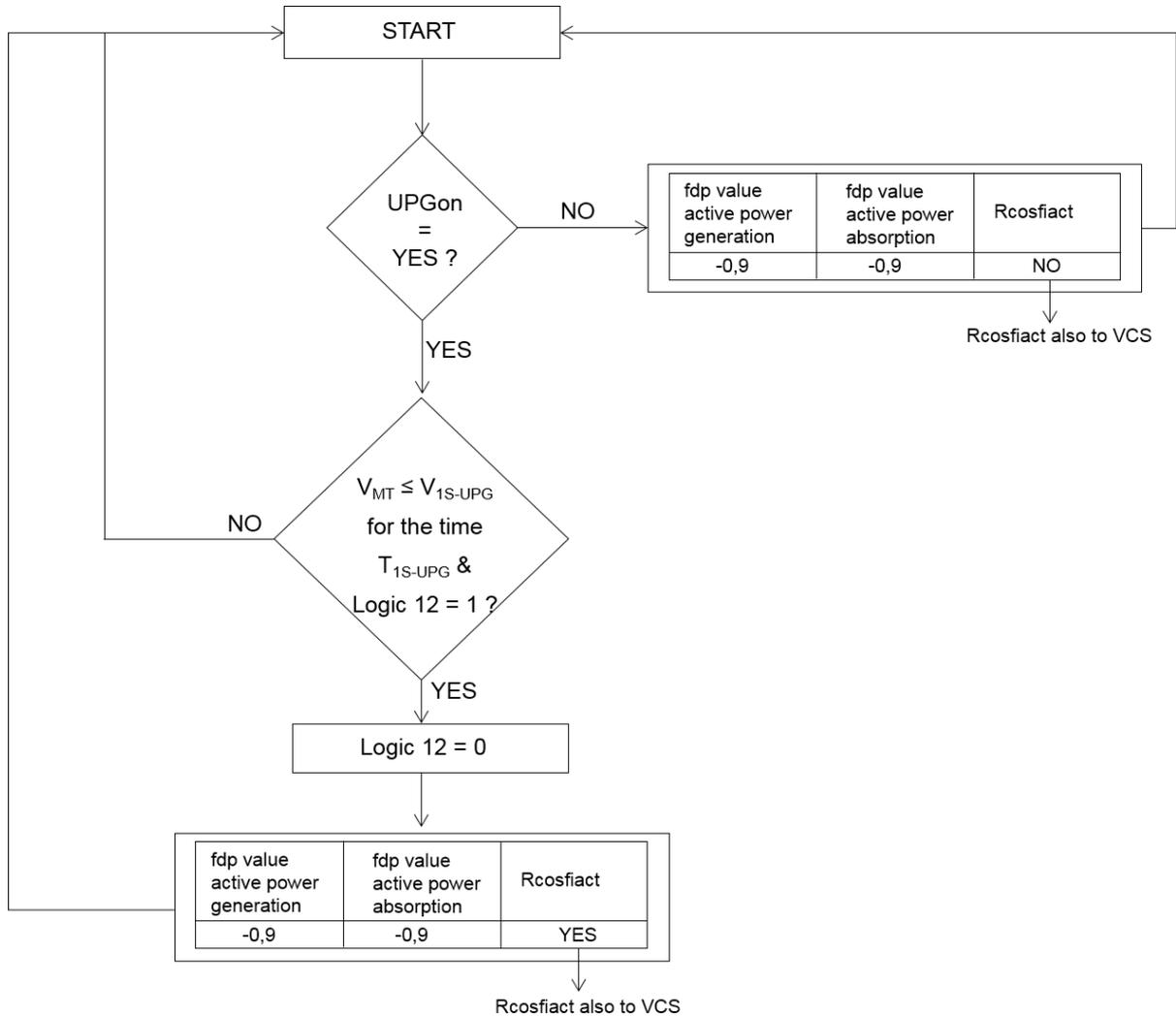
**Figure 5 - Logic for the re-entry of the local absorption of Q (logic 2)**
