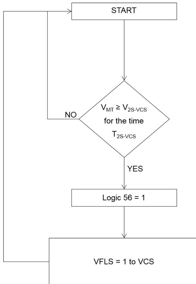
**Figure 8 – Logic for sending VFLS to the VCS (logic 5)**
