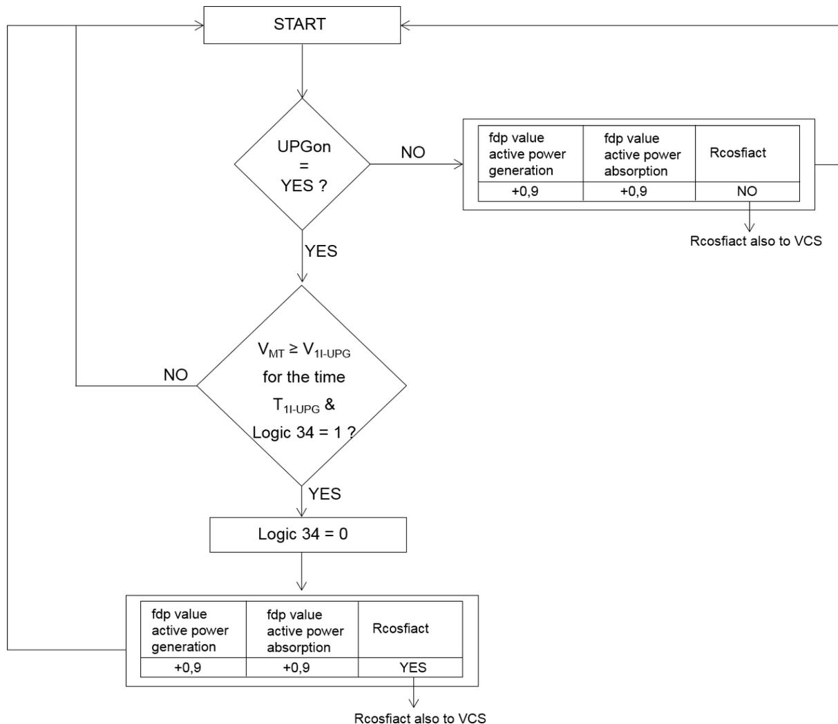
Figure 7 – Logic for the re-entry of the local generation of Q (logic 4)
