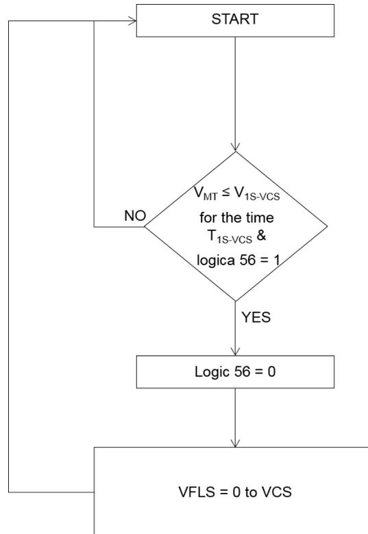
**Figure 9 – Logic for the re-entry of the VFLS to the VCS (logic 6)**
