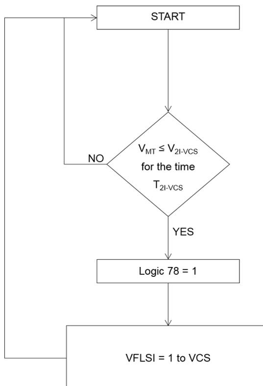
**Figure 10 – logic for sending VFLI to the VCS (logic 7)**
