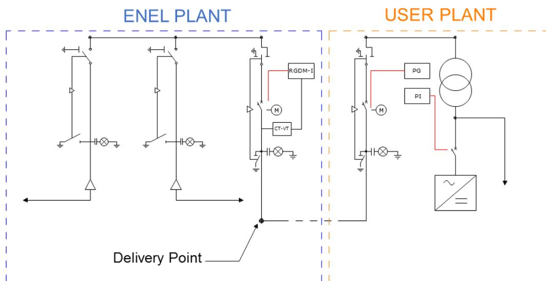
Figure 1 – DG Installation mode
