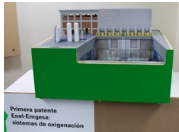
Image 1. Patent Model "Microinjection and oxygen dosing system for discharge water from a hydroelectric plant" Enel Emgesa 2019
